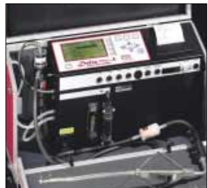
DELTA 1600 L * COMPACT INSTRUMENT for stationary and portable applications - CO · HC · CO 2 · NO · O 2 · Stationary and portable Weight: approx. 10 kg
