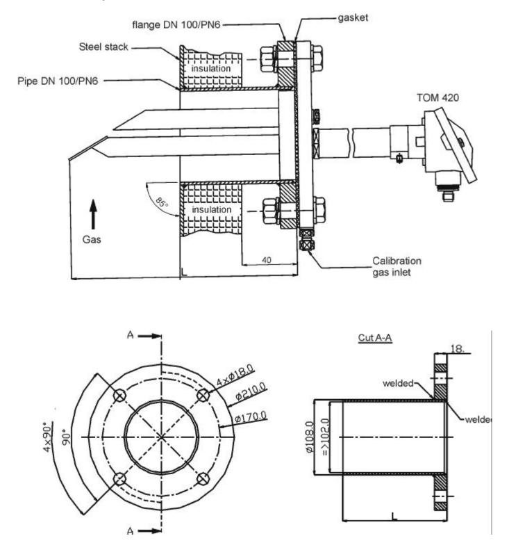
illustration pipe/flange assembly (supplied by customer)
