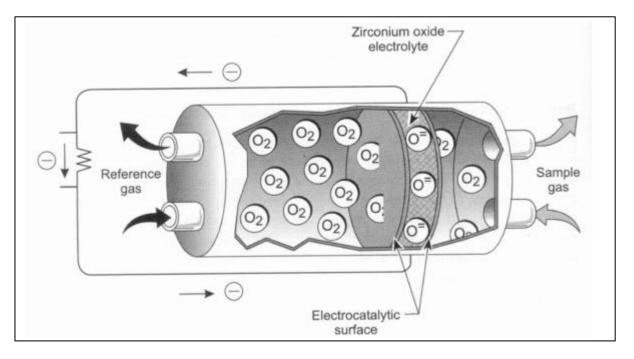
The electro-motive force (emf) that is generated across the solid electrolyte by the passage of oxygen ions, can be measured as a sensor voltage.
